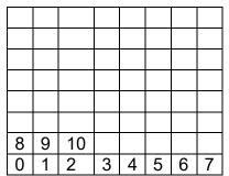
Just you think this block represents as memory. Memory is divided into smaller addressable unit, that is called byte. Let us assume these boxes are bytes. Every byte is having address...address is this 0,1,2,3,4,5,6...like this. Diagram is two dimension but address is single dimension. So, addresses are linear not like coordinate system[x,y].
